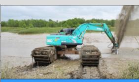
*Engineered options* : Supplementary Pontoons Spud System Expandable Tracks Polymer Tracks
